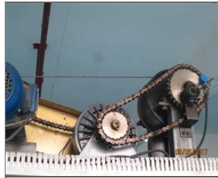
Photo of non-conformity NC 7.17 No safety guard.JPG
